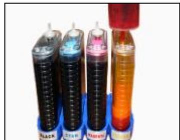
Please kindly to take care of the ink level in the reservoirs, if the ink level is below 1CM from the bottom, it alarms you need to refill the ink duly. Carefully pull out the rubber plugs on the refill holes.(Avoid the ink will spattering out )Refill in the according inkjet ink, wipe the refill hole and rubber plug to keep the clean of it
