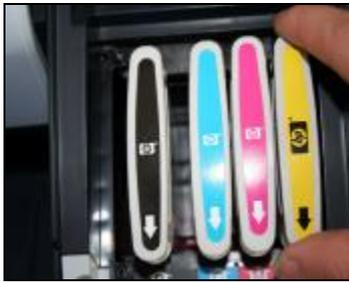
Remove out the original cartridges
